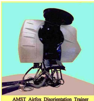
They have full yaw freedom and can produce low-rate motion below the pilot's vestibular threshold.
