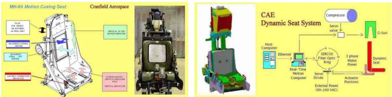
**H8.1 Seat pressure pad.** This gives an effective cue of seat pressure under G, particularly for the lower G values before G-suit onset. I have also flown a simulator with multiple seat pads with different inputs, but these are complex, expensive, can give confusing cues, and are not recommended.
